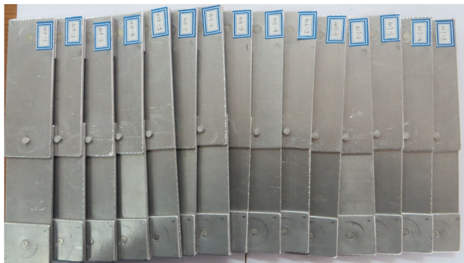
Figure 4. Material drawing after riveting of shear test piece
