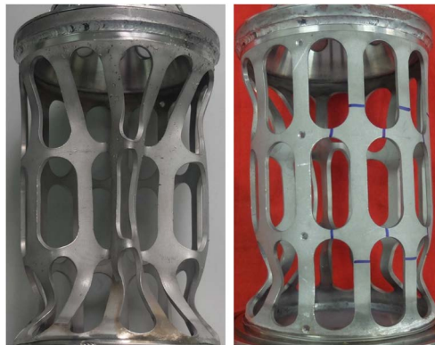
Figure 4. The destroy of filter skeleton
