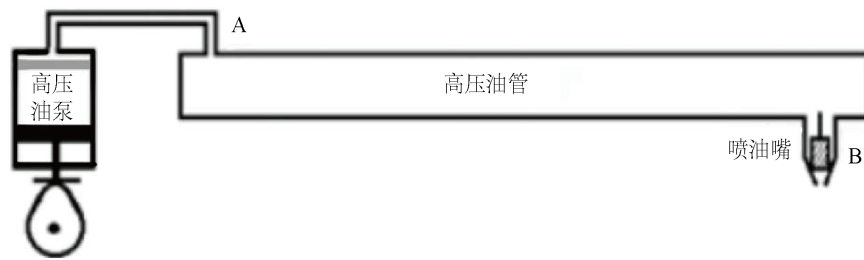
Figure 1. High pressure tubing model in actual working process
