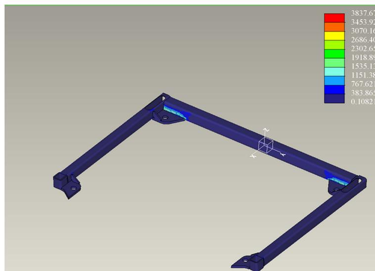
Figure 9. Cab support static loading analysis
