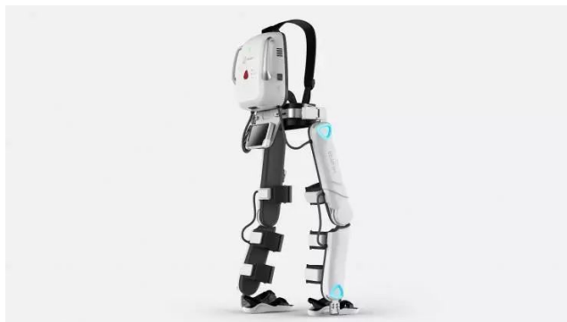
Figure 1. Exoskeleton robot BEAR H1 based on flexible drives
