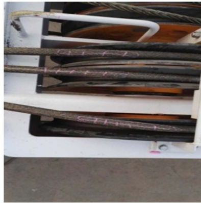
Figure 5. Marking of wire rope joint 图 5. 钢丝绳琵琶头标记
