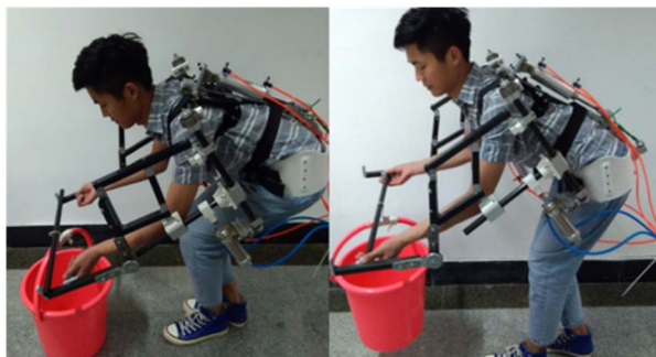
Figure 9. Test prototype of wearable handling assistance robot 图 9. 可穿戴搬运助力机器人试验样机
