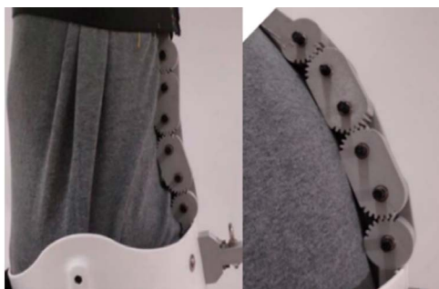
Figure 5. Diagram of multi-axis single degree of freedom mechanism wearing 图 5. 多轴单自由度机构穿戴示意图
