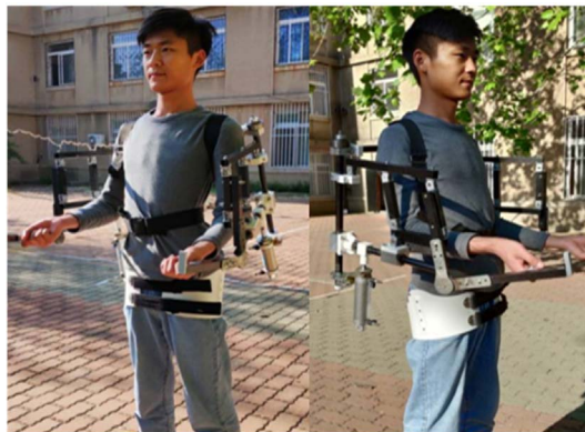
Figure 8. Test prototype of wearable handling assistance robot 图 8. 可穿戴搬运助力机器人试验样机
