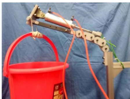
Figure 10. Power-assisted experiment of multi-axis single-degree-of-freedom 图 10. 多轴单自由度助力实验
