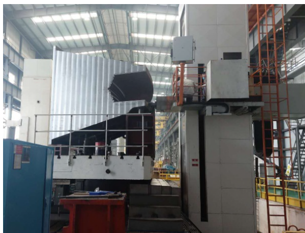
Figure 4. The actual situation of the main cable saddle cable groove processing 图 4. 主索鞍鞍索槽加工实物情况
