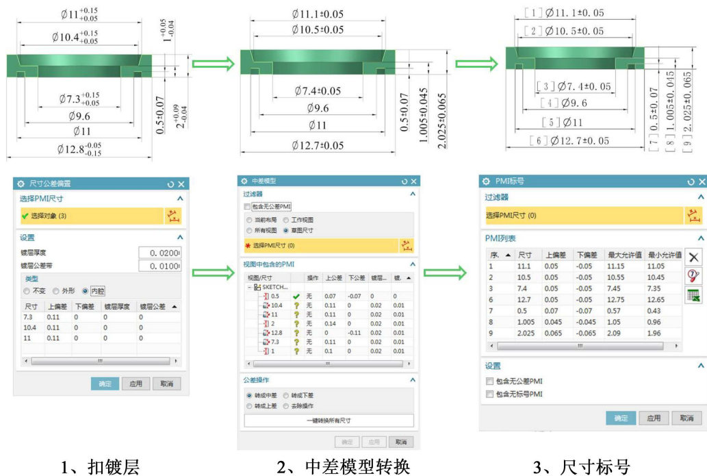
Figure 3. Legend of MBD process model conversion steps 图 3. MBD 工艺模型转换步骤图例
