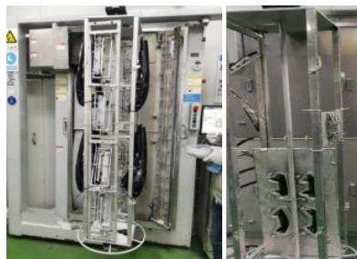
Figure 6. High vacuum aluminizing unit 图 6. 高真空镀铝装置
