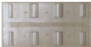
Figure 4. Injection molded parts (PC)
