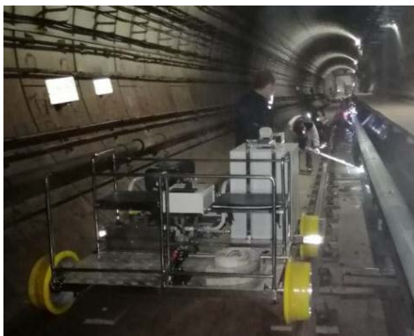
Figure 12. Prototype test of combined metro track electric trolley 图 12. 组合式地铁轨道电动小车样机试验
