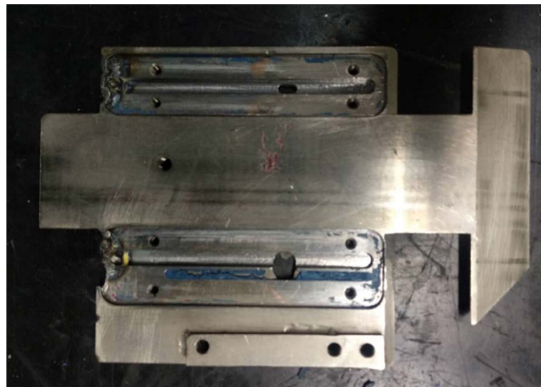
Figure 3. Suction chamber for negative pressure suction module with lining paper 图 3. 内衬纸负压吸风组件吸风室实物图
