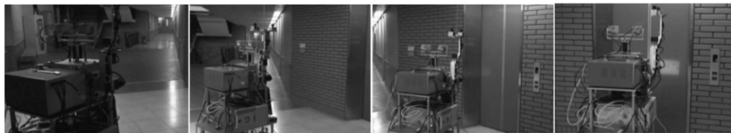
Figure 13. Robot recognition elevator bearing process 图 13. 机器人识别电梯方位过程
