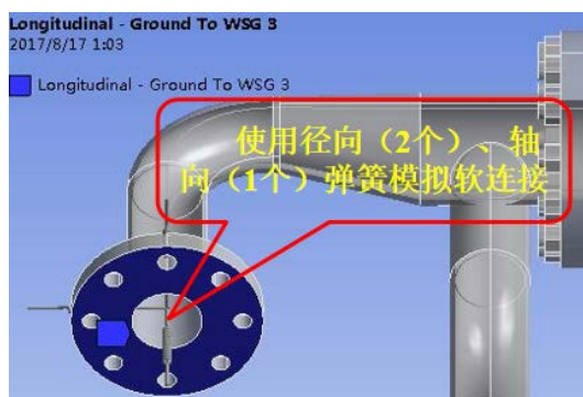
Figure 14. Boundary condition diagram after adding soft connections 图 14. 加软连接后边界条件
