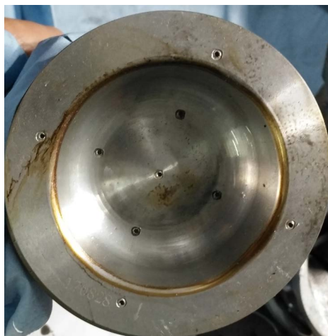
Figure 11. Piston installed with hardness plug 图 11. 安装硬度塞后的活塞
