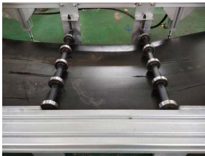
Figure 7. Vibration damping device and its installation layout diagram 图 7. 减振装置及其安装布局图
