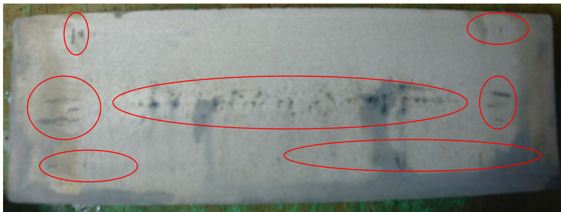
Figure 6. The low times shown billet before transformation 图 6. 改造前带钢坯低倍图示
