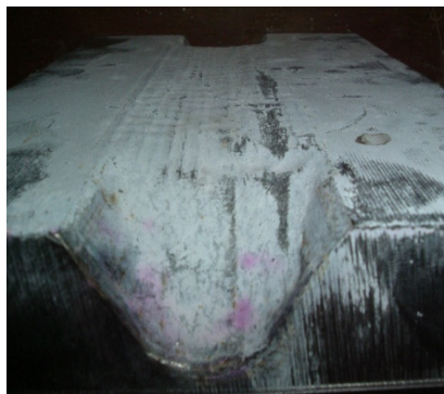
Figure 3. Samples for laser cladding repair
