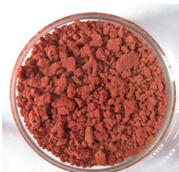
Figure 3. Macroscopic morphology of electrolytic copper powder
