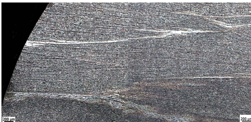
Figure 3. Microstructure of sample segregation zone 图 3. 试样偏析带组织
