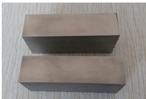
Figure 1. Diagrammatic of diffusion bonded samples
