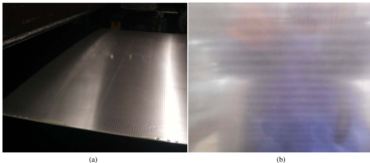
Figure 1. Vibration marks defect. (a) Overall morphology of defect on rolling; (b) Overall morphology of defect after degreased
