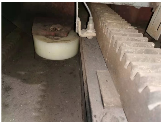
Figure 6. Physical drawing of buffer wheel and rack position diagram 图 6. 缓冲轮和齿条位置实物图
