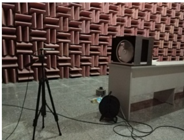
Figure 10. Axial fan noise test
