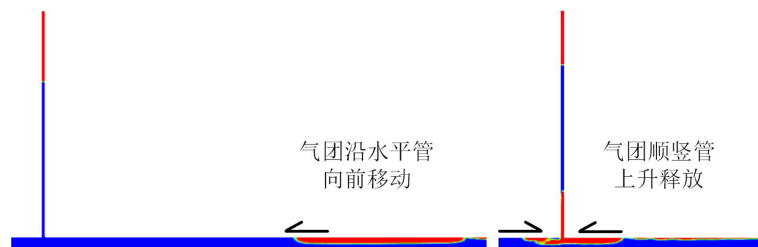
Figure 3. Working condition (Bd) simplified gas-liquid phase cloud diagram with constant diameter ratio
