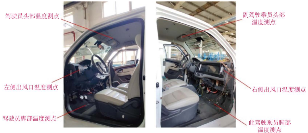
Figure 7. Schematic diagram of the temperature measurement point inside the car 图 7. 车内温度测点位置示意图
