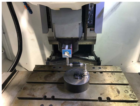
Figure 7. Experimental site diagram of double ball bar instrument 图 7. 球杆仪实验现场图
