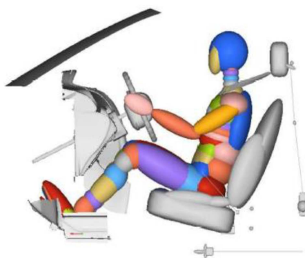
Figure 6. Simulation model of driver restraint system model 图 6. 驾驶员约束系统仿真模型
