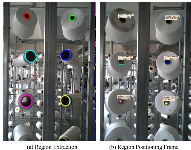
Figure 11. Contour extraction and positioning result of yarn bobbin. (a) Yarn bobbin area extraction. (b) Yarn bobbin positioning frame. 图 11. 纱筒轮廓提取及定位效果。(a) 纱筒区域提取; (b) 纱筒定位框
