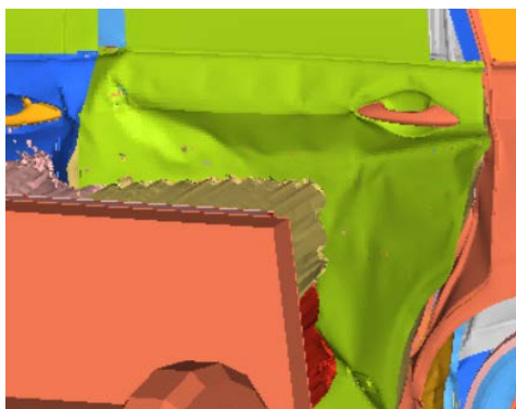
Figure 4. Deformation diagram of door panel 图 4. 车门外板变形图
