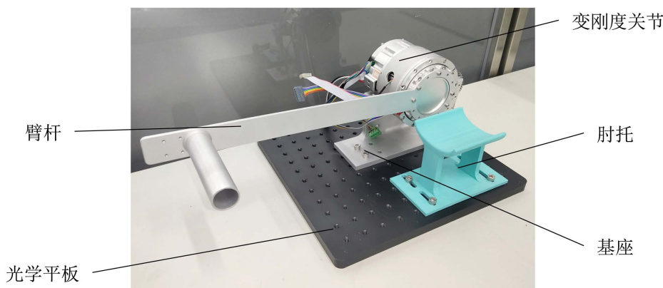
Figure 2. Variable stiffness elbow joint rehabilitation robot platform 图 2. 变刚度肘关节康复机器人平台
