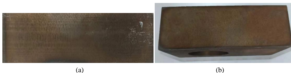
Figure 10. Workpiece surface after thermal energy deburring 图 10. 热能去毛刺后工件表面
