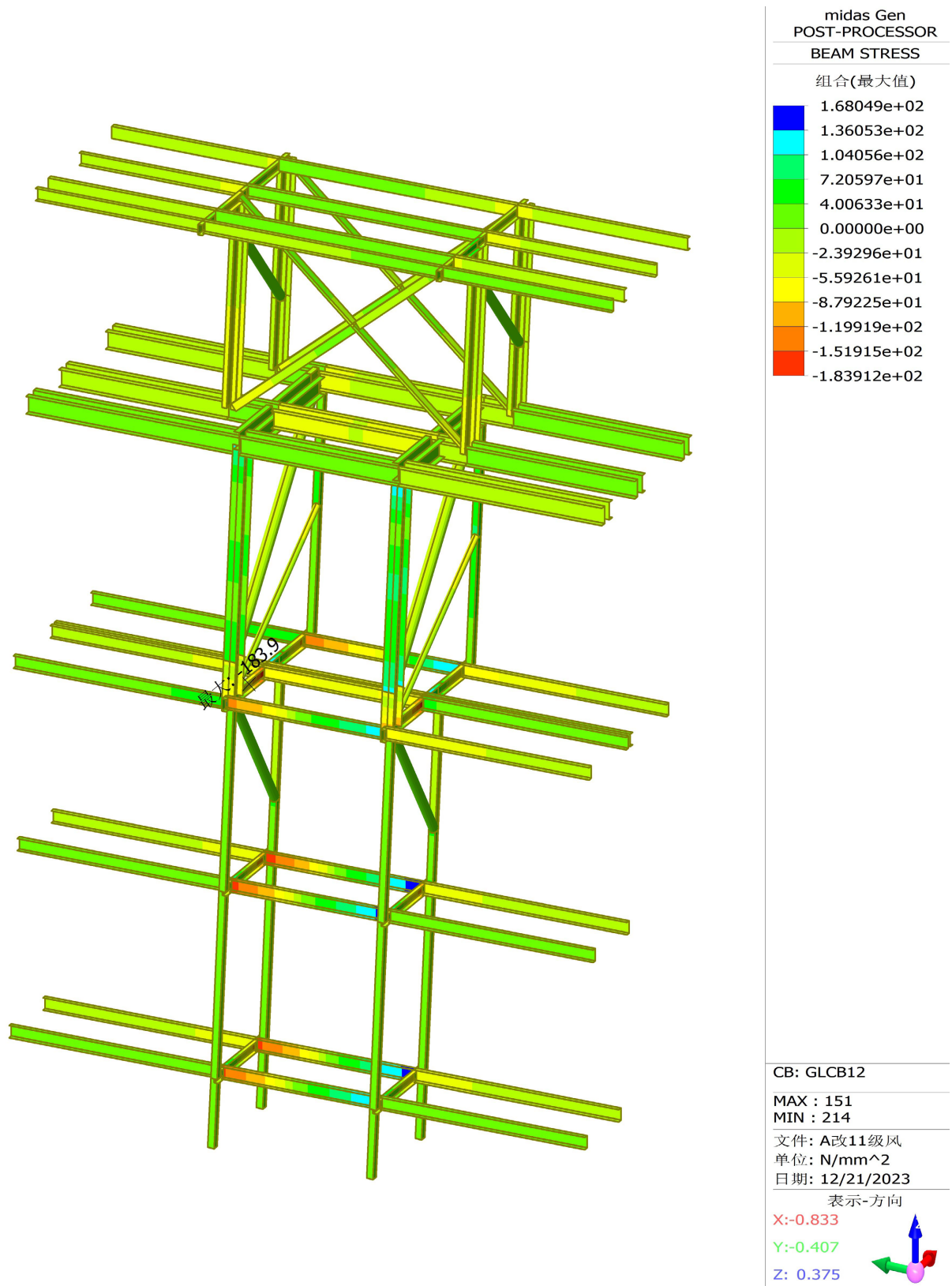
Figure 8. Structural stress diagram under working condition III 图 8. 工况三下的结构应力图
