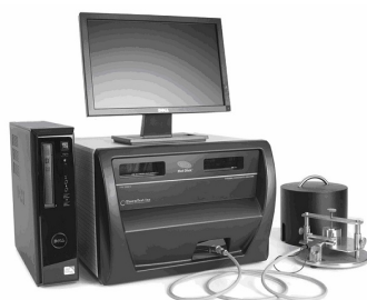
Figure 1. Thermal constant analyzer (Hot Disk TPS2500S) 图 1. Hot Disk TPS2500S 热常数分析仪
