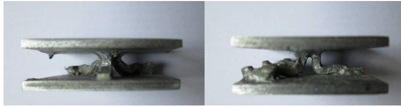
Figure 4. The completely crushed tetrahedral lattice truss sub-element 图 4. 压缩完成后的正四面体点阵夹芯单体图
