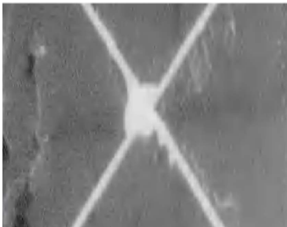
Figure 2. The row lattice method test pattern of 1 sample 图 2. 1#样品划格法测试图
