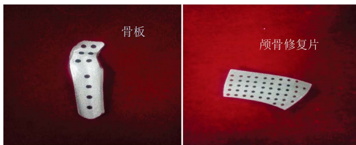
Figure 2. Bone plate and skull repair slice of titanium alloy 图 2. 钛合金骨板与颅骨修复片
