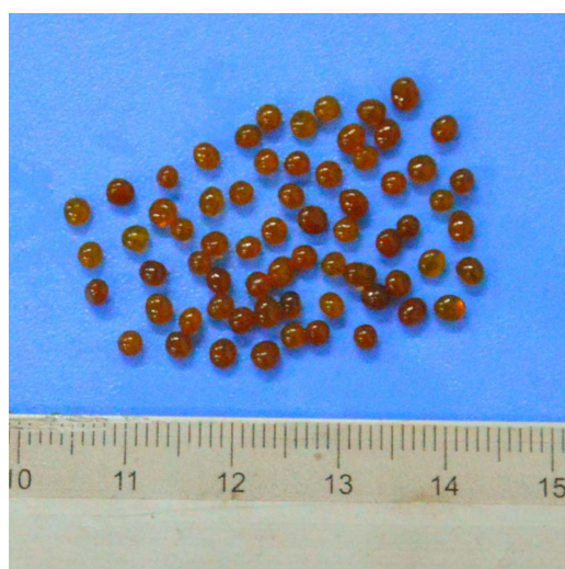
Figure 2. Appearance of the pore former of sugar spheres
