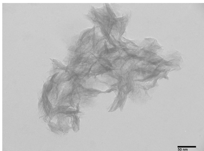
Figure 2. TEM images of the \text{TiO}_2(\text{B}) nanosheets. Scale bar: 50 nm
