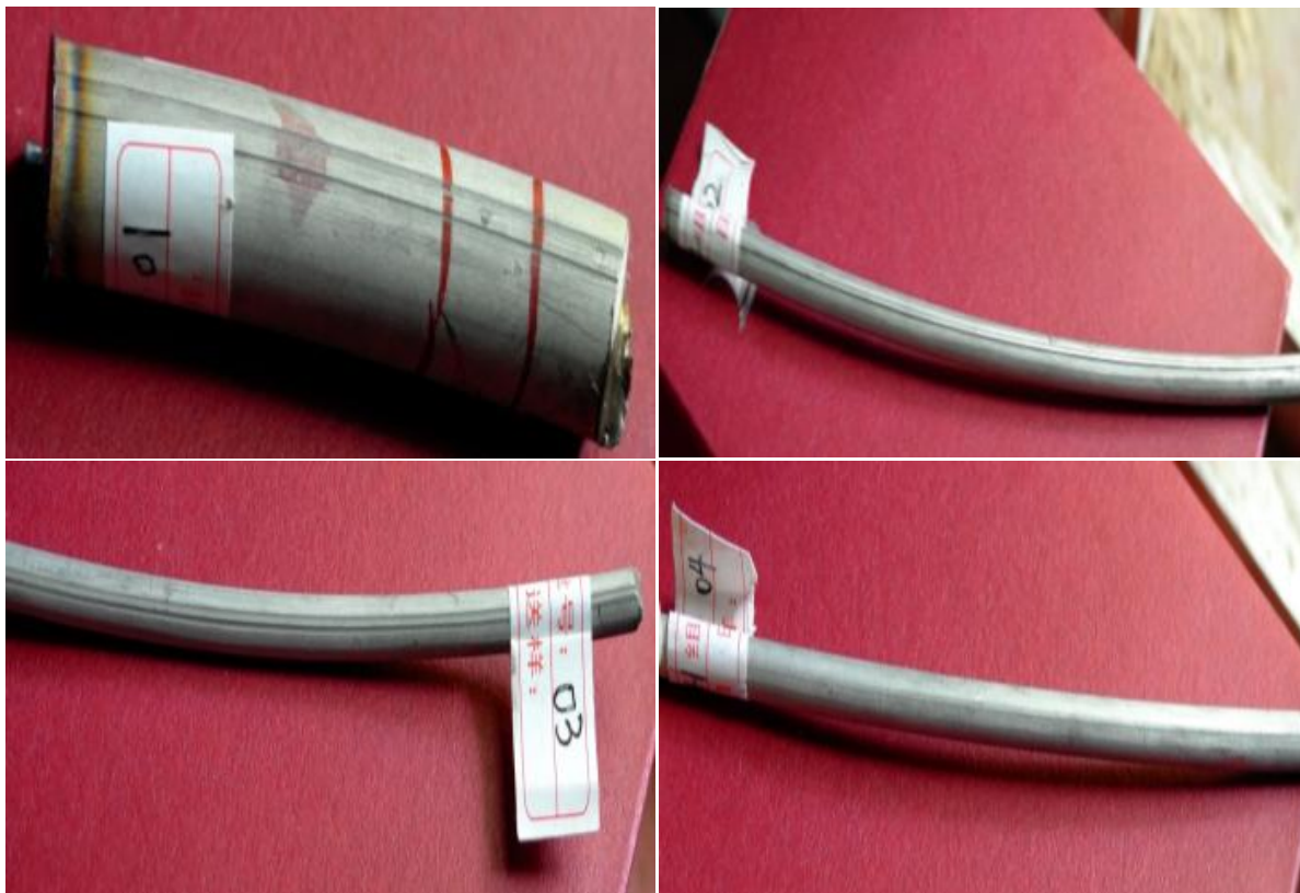
Figure 1. The Macroscopic appearance of black line defect 图 1. 黑线缺陷宏观形貌
