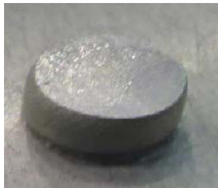
Figure 5. Upsetting tip tipping trend diagram 图 5. 镦头“倾倒趋势”图
