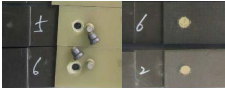
Figure 6. Typical failure mode of single nail and single shear 图 6. 单钉单剪典型失效模式
