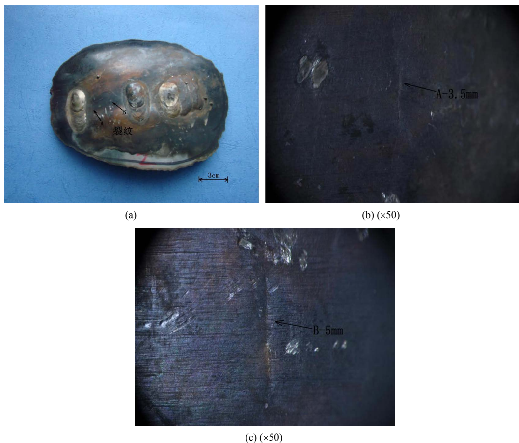
Figure 1. Macroscopic morphology of cracks on the surface of alkali solution filter 图 1. 碱液过滤器表面裂纹宏观形貌
