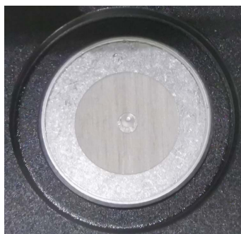
Figure 5. Pole state after laser cleaning
