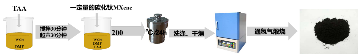
Figure 1. Synthesis diagram of \text{WS}_2 /Titanium carbide MXene nanocomposites
