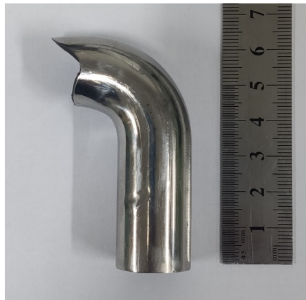
Figure 4. Titanium alloy tube with small bending radius of 0.9 D 图 4. 0.9 D 小弯曲半径钛合金管
