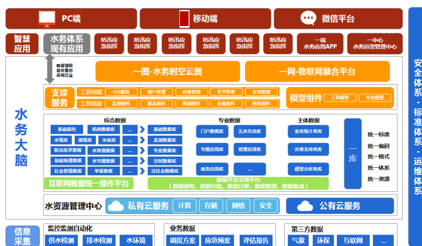
Figure 1. Design drawing of technical framework of a smart water system
