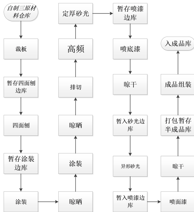
Figure 1. Flow chart of painting frame 图 1. 喷漆像框流程图
