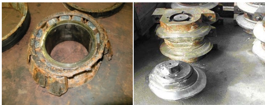
Figure 5. Bearing damage (left) and cutter ring eccentric wear (right)
