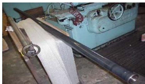
Figure 11. Two US Navy submarine parts thermal sprayed with nanostructured ceramic coatings
